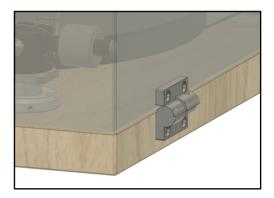
The new design also provides a stop point at about  $90^{\circ}$  to the dust cover: in this position it automatically stops and the hinges will hold the dust cover avoiding overturning.
